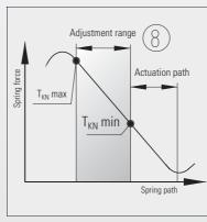
Attention! R+W safety couplings have disc springs with a special characteristic. The torque adjustment range lies within a specific range of positions for the disc spring, outside of which the torque limiter can not function. It is important to always stay within the min. – max. of the specified torque adjustment range.
