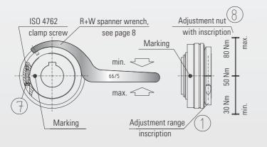
R+W safety couplings are preset and marked with the desired disengagement torque setting at the factory. The min. and max. of the torque adjustment range are then also marked on the adjustment nut (1). Disengagement torque is continuously adjustable within the range (8) though adjustment of the tension on the disc springs.
