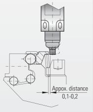
The switch's plunger should be positioned
